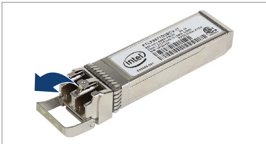
Figure 39: Unlatching the locking bail
